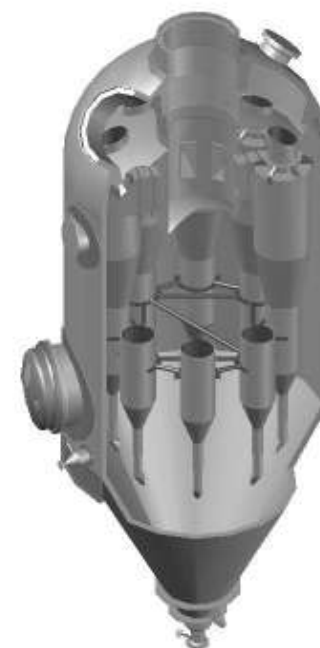
Third Stage Separator (TSS) Cutaway
