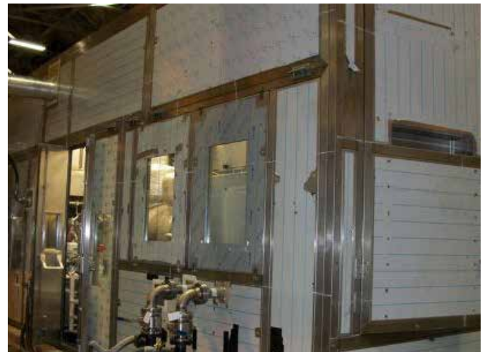
Pump acoustic enclosure on test.
