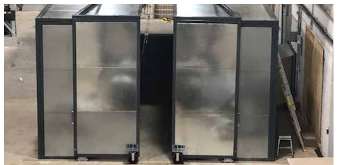
Blast cleaning enclosure.
