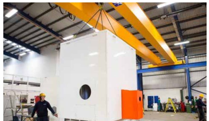
Ventilated acoustic enclosure for a large blower for a petrochemical client.
