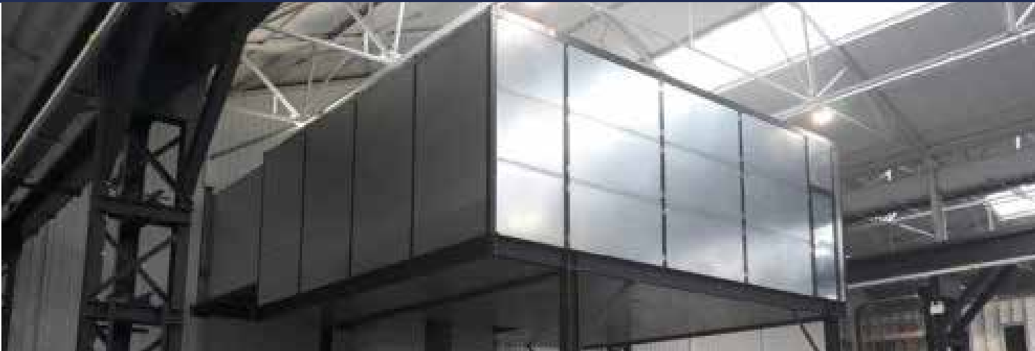
Acoustic enclosures and acoustic rooms for manufacturing equipment and processes.
