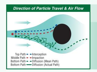
Particles are collected by a combination of mechanisms: impaction, interception and Brownian Diffusion. Collection of particles less than 2 microns is primarily due to Brownian diffusion; a collection mechanism somewhat unique to the fiber bed filter.
