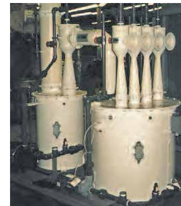
ET Series Multi-stage ejector tower toxic gas scrubber
