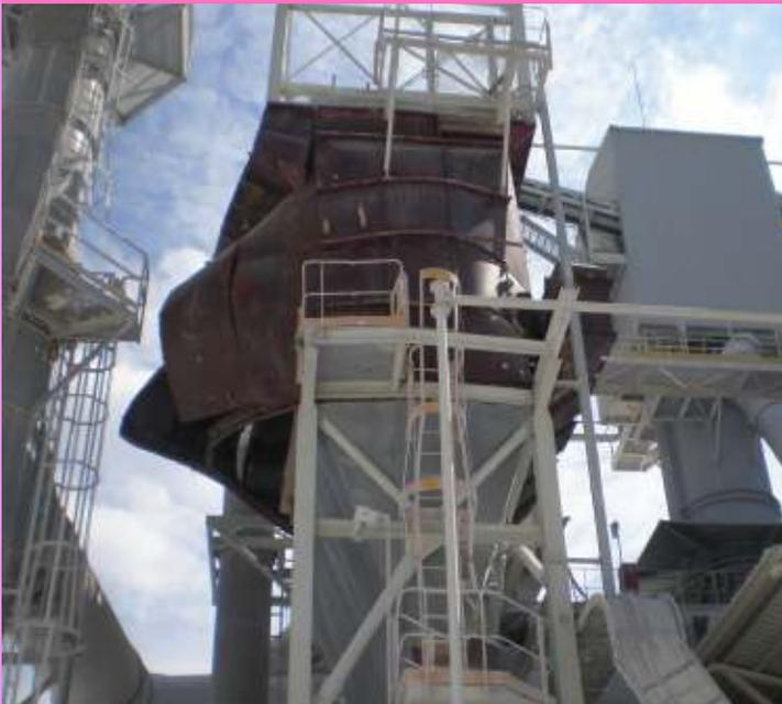
The original dust collector included 300 filters, featured panelized construction, and was fabricated in Austria and assembled on site with hopper heat tracing and insulation.
