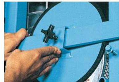
Notched end of the horizontal bar slides over studs, aligning the gasketed clamp over the filter end cap. All cartridge gasket surfaces mate perfectly every time.
