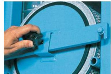
Unique toggle screw handle allows for proper compression of sealing gaskets and perfect alignment of cartridges every time.
