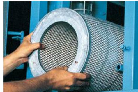
The cdc™ cartridges slide easily in and out of the collector. Support rails guarantee perfect cartridge alignment every time.
