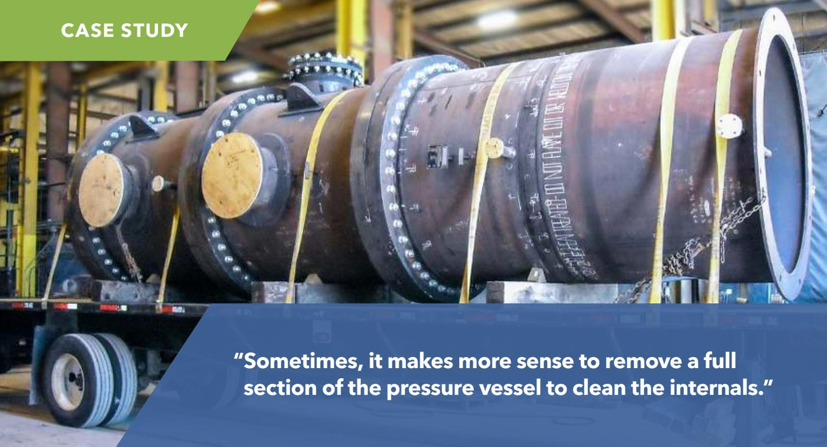
**“Sometimes, it makes more sense to remove a full section of the pressure vessel to clean the internals.”**
