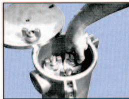
3. Unscrew filter tube cap nuts.
