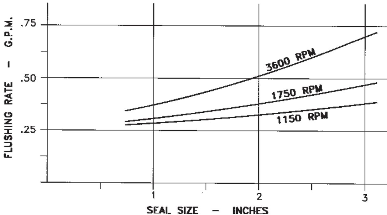
FLUSH PRESSURE - 15 TO 25 PSI ABOVE STUFFING BOX PRESSURE
