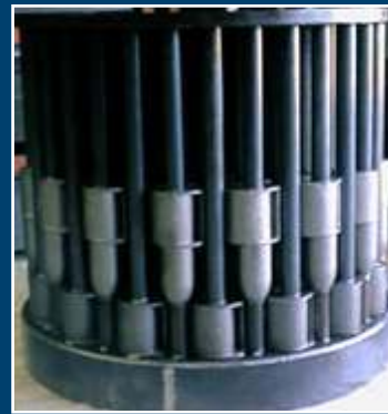
Multi-cyclone separation internals used for the removal of solid and liquid contaminants within a vertical pressure vessel. This “dense pack” configuration is designed for handling intermittent liquid slugs.
