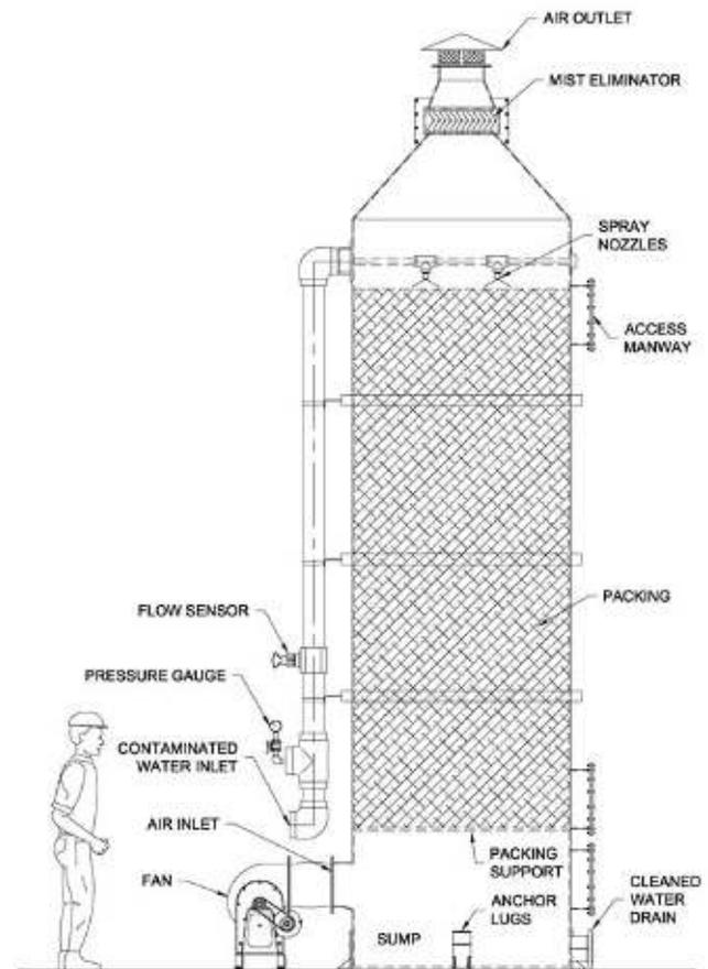
HEE's Air Stripper Towers Model HAST are complete cylindrical towers filled with a high efficiency packing, mist eliminator, liquid distribution system, access man ways, an integral sump with a flat bottom, and a blower. The Air Stripper Tower Model HAST can accommodate a wide range of contaminant concentrations and liquid flow rates. The towers and internal components are fabricated using corrosion resistant materials such as fiberglass reinforced plastic (FRP), polypropylene, and PVC.
