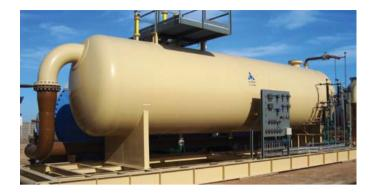
The layer of separated oil flows at a constant rate over a fixed weir into the recovered oil sump from where it can be released intermittently during the process via a level switch controlled valve. The treated water leaves the separator vessel via the control valve an can be further treated if required by floatation or filtration.
