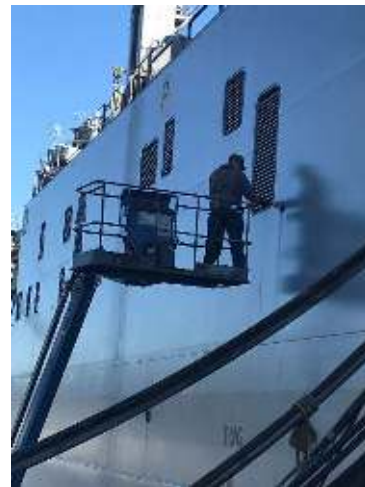
Figure 15: Shiplside access to work on louvers requires a hydraulic lift platform and associated ground crew aboard USN Charles Drew (T-AKE-10)
