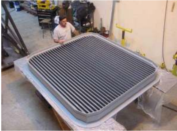
Figure 9: Assembly of a "large" LPD louver before installing FOD screen and drilling mounting bolt holes
