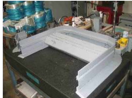
Figure 7: “Dry-Fit” pre-assembly of LPD louvers to confirm parts fit-up
