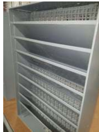
Figure 12: Back side of T-AKE louver depicting vane blades and composite FOD grating
