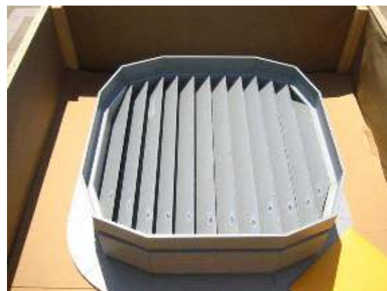
Figure 8: Assembly of a “small” LPD louver before installing FOD screen and drilling mounting bolt holes
