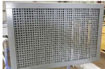
Figure 13: Front side of T-AKE louver showing composite FOD grating and square cornered frame
