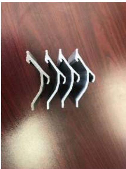
Figure 18: FRP pultruded moisture separator vanes (Peerless P2-XLP-C profile)
