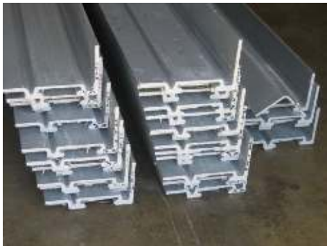
Figure 5b: Lengths of LPD louver frame parts depict the uniform cross section grooves
