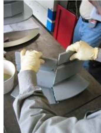
Figure 6: Tongue-and-groove assembly of LPD louver frame radiused corner with epoxy adhesive
