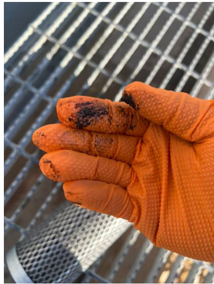
Figure 4 – Solid Black Debris Recovered from Amine Regeneration System
