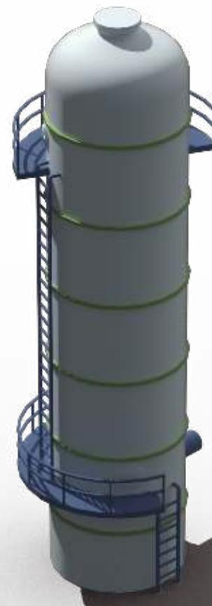
it gets heated by exchanging heat with the heating source passing through reboiler tubes. The heating results in separation of volatile hydrocarbons and H<sub>2</sub>S from crude oil making crude stable and sweet. The stabilized crude leaves the column from the bottom and gets cooled in the crude pre-heater before flowing to storage tanks.
