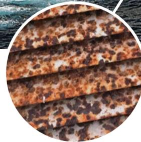
Corrosion is constantly occurring aboard U.S. Navy vessels resulting in unsightly effects. To address this environmental challenge, several different manufacturing techniques have been developed to apply FRP materials for air intake moisture separators and shipside louvers.
