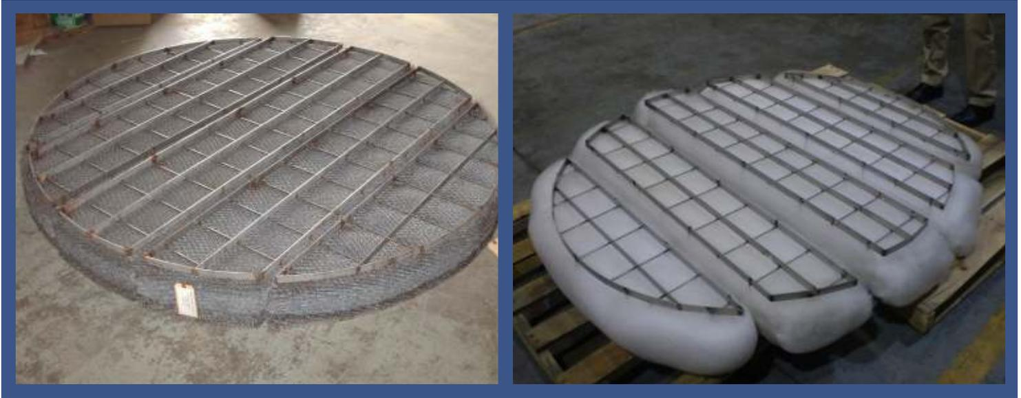
We use co-knitted wire mesh configuration to enhance mist eliminators capabilities. We can knit additional fibers in conjunction with the standard wire to achieve higher surface area and in turn, higher efficiency. These additional fibers promote coalescing of droplets and achieve fine droplet removal.
