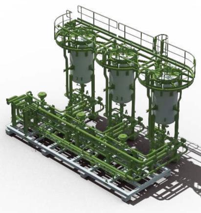
The Walnut Shell Filter performs at its best in produced water applications where outlet requirements are very strict. Not only does the Walnut shell have the ability to act as a fine filter, but the shells themselves coalesce the oil droplets within the media allowing greater efficiency in the removal.
