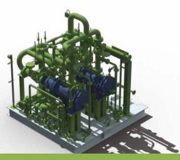
Hydrocyclones are effectively centrifugal separators that rely on the differential density between the oil droplet and the water to allow separation. **The efficiency** of the separation is governed by five main factors:
