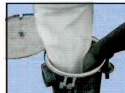
Remove filter bag from chamber.
