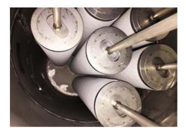
maximize droplet formation and disengagement. Small liquid droplets suspended in the continuous phase come together, or coalesce, as the mixture moves through the coalescer medium.
