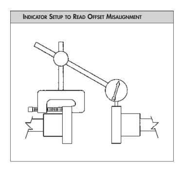
To check the offset alignment, mount the dial indicator as above except with the indicator button on an outside diameter of the stationary coupling hub. Rotate the shaft on which the dial indicator is mounted, allowing the indicator button to ride on the outside diameter of the stationary hub. The indicator dial movement will show the difference in the center locations of the two shafts. Good practice suggests alignment to within 0.002" T.I.R.
