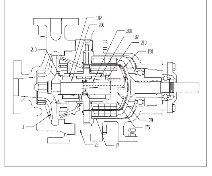
The internal circulation flow path through the bearings and the magnetic coupling is supplied with discharge pressure and returns to discharge pressure. The differential pressure required to do this is supplied by an impeller built into the outer end of the inner magnet assembly (175). This flow provides cooling to the magnets (175) and the containment shell (150) and also lubrication as well as cooling to the bearings (182), journal sleeves (200) and thrust collars (210).
