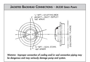
WARNING — EXTREME HAZARD TO PERSONNEL: Improper connection of cooling water piping may result in the injection of cooling water into the pump stuffing box and into the pumpage. Depending on temperature this may cause a violent steam explosion in the pump, piping, or associated equipment with extreme hazard to personnel. It may also cause serious contamination of the pumpage and heavy corrosion of pump or equipment parts.
