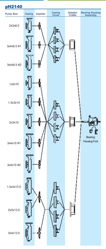
Casing covers with jackets, standard bore, large taper bore, and large cylindrical bore seal cavities are available on all pumps. Bearing housings with finned tube oil coolers are also available on all pumps.
