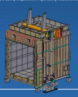
the HRSG to gradually come online. This approach offers the flexibility of fast power and increases the life of an HRSG. In todays business environment bypass exhaust systems provide a solution for the option between baseload and peaking/modulating operation.
