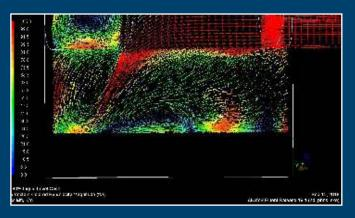
CFD flow patterns at original (high) liquid level indicate scooping action which re-entrains liquids. [Red = high velocity; Blue = low velocity
