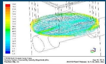
CFD flow patterns at optimized (lower) liquid level approach the four-bank vane unit uniformly after passing the  $\frac{1}{2}$  pipe baffle.
