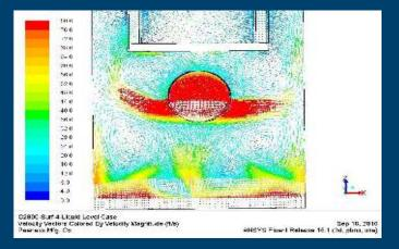
CFD flow patterns at optimized (lower) liquid level confirm the gas flow passing around the inlet ½ pipe baffle.
