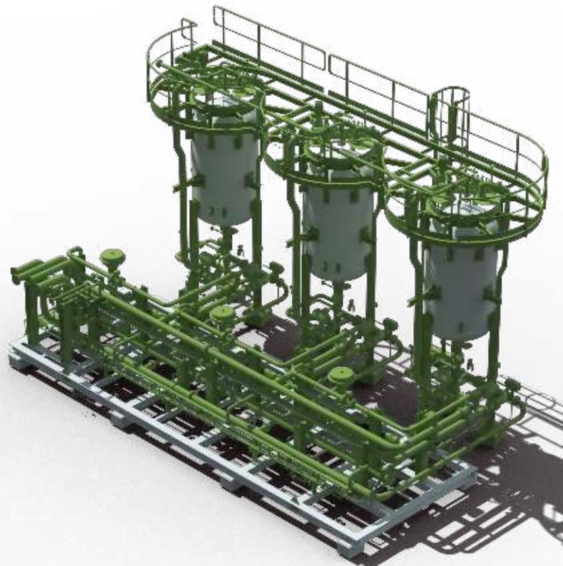
The Walnut Shell Filter performs at its best in produced water applications where outlet requirements are very strict. Not only does the Walnut shell have the ability to act as a fine filter, but the shells themselves coalesce the oil droplets within the media allowing greater efficiency in the removal.
