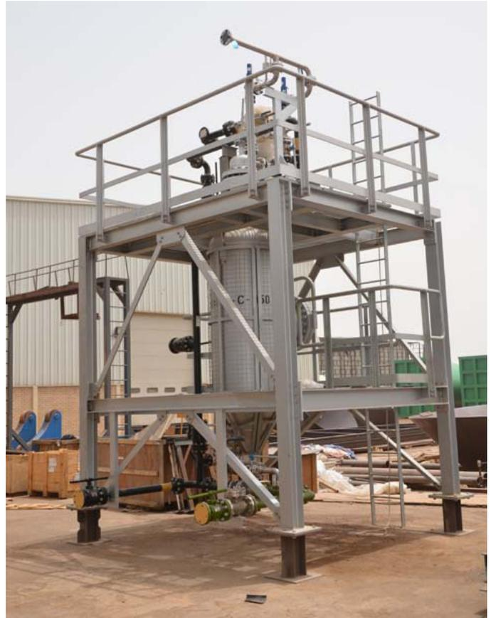
During sand washing the vessel is isolated from the upstream separators, wash water is used to recirculate the accumulated solids through the desanding hydrocyclone liners.
