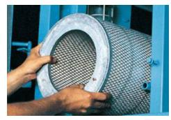
The **cdc™** cartridges slide easily in and out of the collector. Support rails guarantee perfect cartridge alignment every time.
