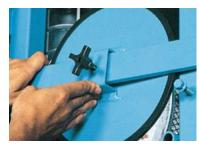
Notched end of the horizontal bar slides over studs, aligning the gasketed clamp over the filter end cap. All cartridge gasket surfaces mate perfectly every time.
