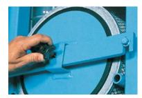
Unique toggle screw handle allows for proper compression of sealing gaskets and perfect alignment of cartridges every time.
